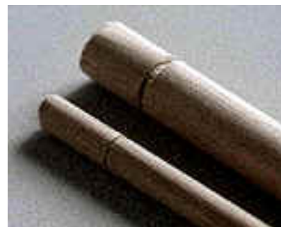
Close up of cut in the dowel to keep the line from slipping off
